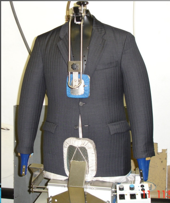
Tensioning Form Finisher
